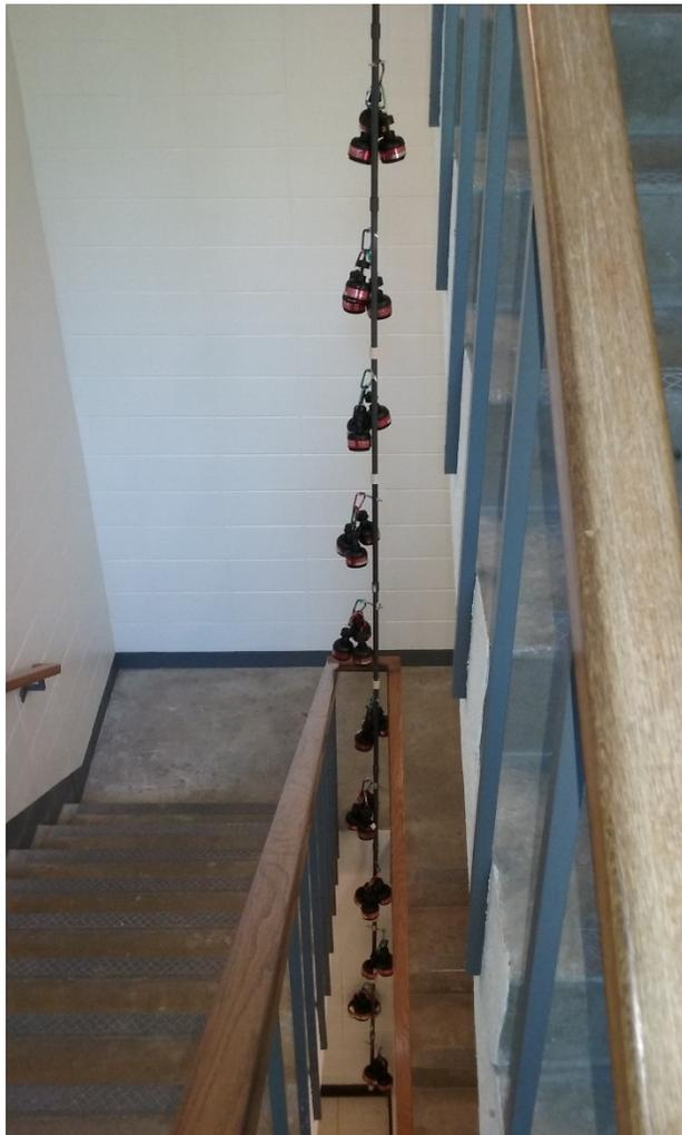
Figure (9): Indoor radon tower.
