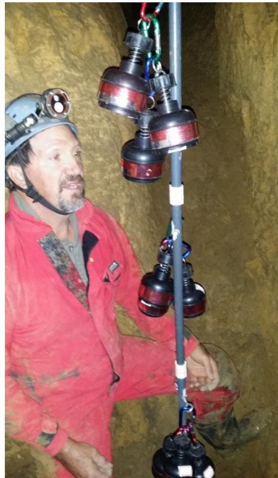
Figure (12): Kemling Cave internal radon tower construction.
