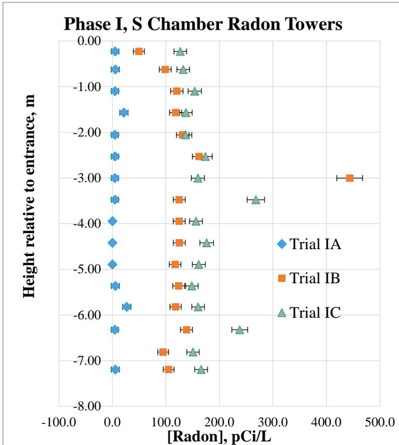
Figure (4): Phase I, S chamber radon towers
