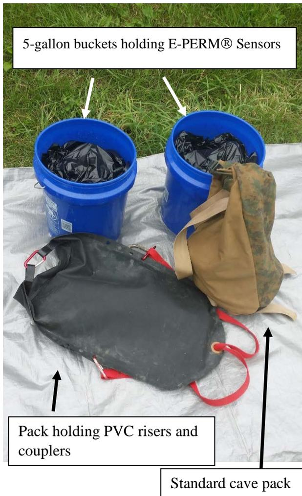
Figure (11): Kemling Cave internal radon Tower components ready for transport.
