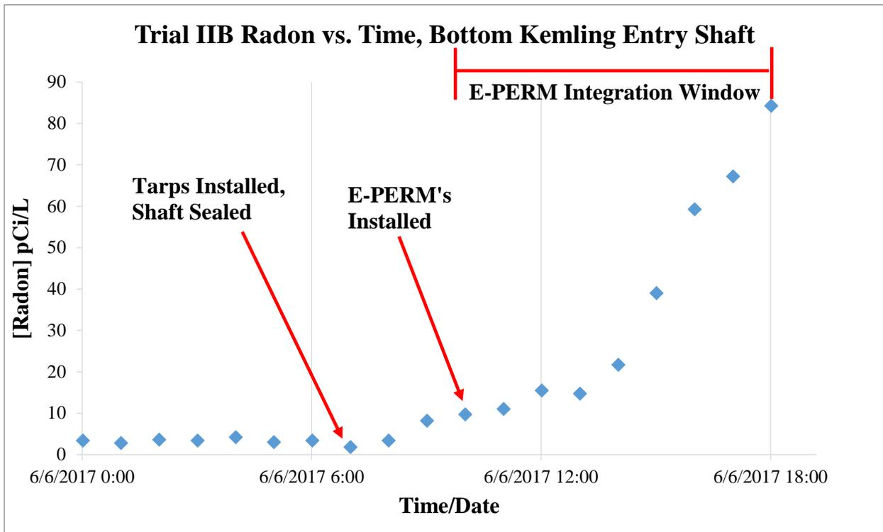
Figure (6): Radon change over time during Trial IIB.
