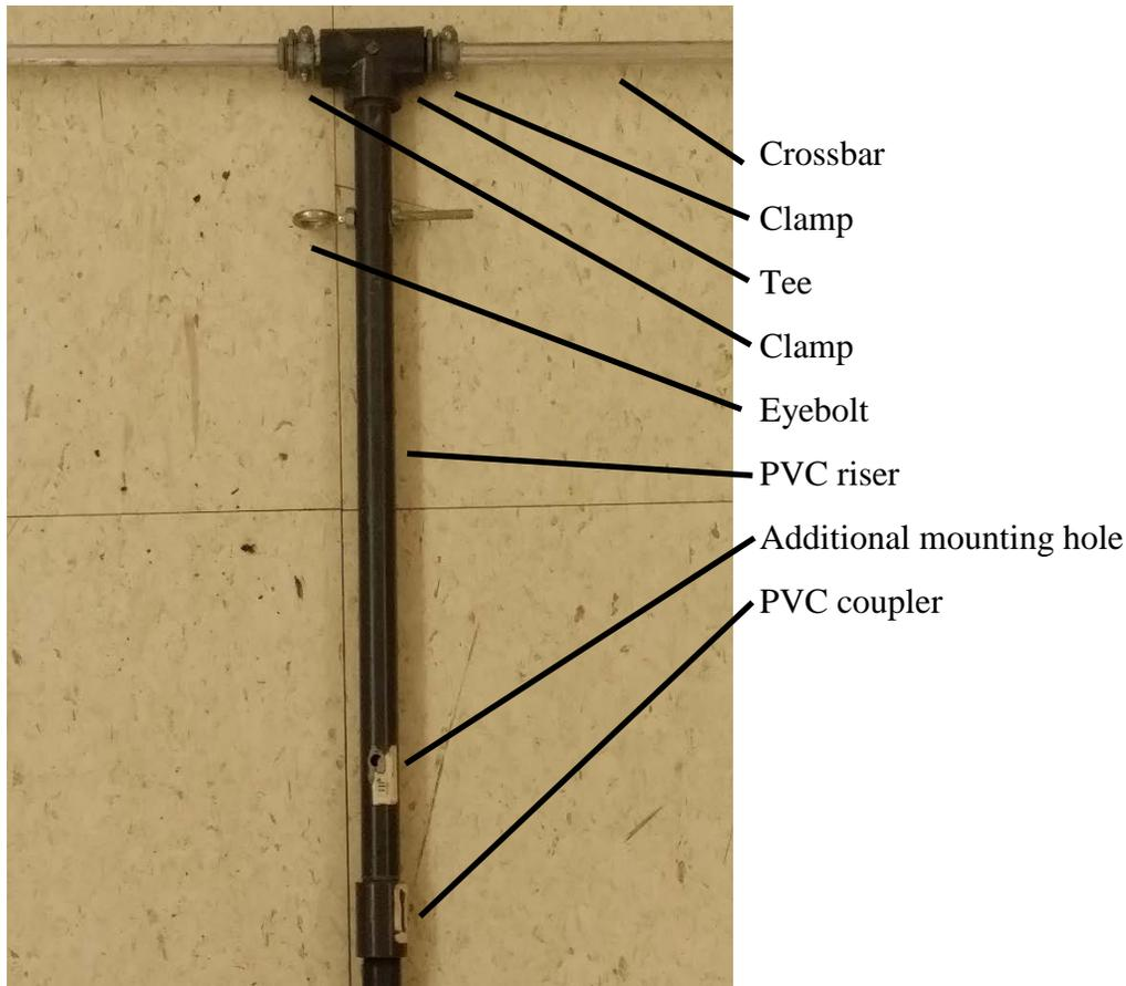
Figure (2): Segments of the radon tower.
