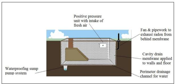
Figure (12) Illustration of components used in combined basement waterproofing and radon management system
