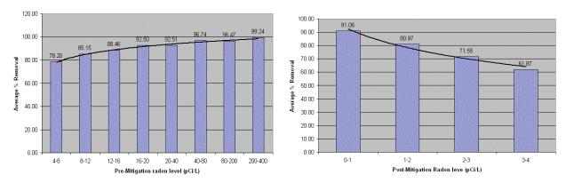
Figure 3: Variation of Removal Efficiency with Pre-Mitigation and Post-Mitigation Levels for the Best Performing System for Year 2008
