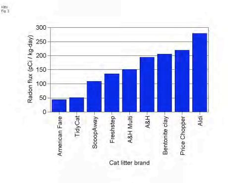
Fig. 3. Radon flux results of the measured samples of cat litter and bentonite clay.
