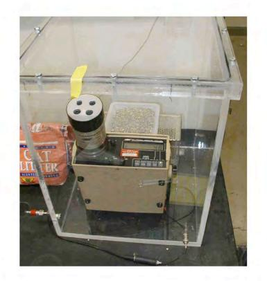
Fig.1. Photograph of the radon detection system used in the analysis of the cat litters.
