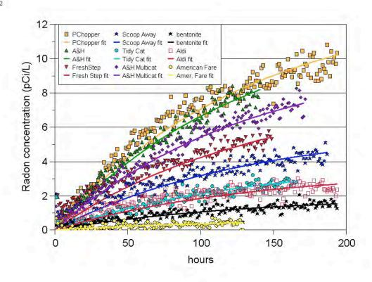
Fig. 2. Radon activities determined in samples of cat litters and bentonite clay. The solid lines represent the expected activities based on the 3.82-d half-life of radon.
