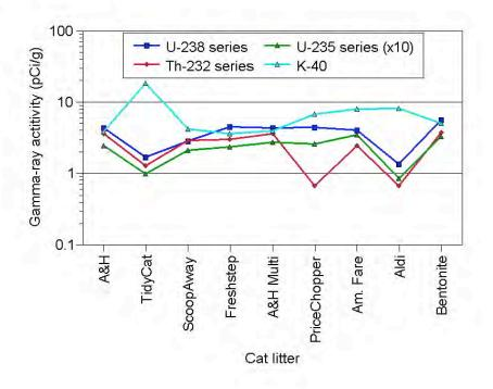
Fig. 4. Gamma-ray activities determined in samples of cat litter and bentonite clay.
