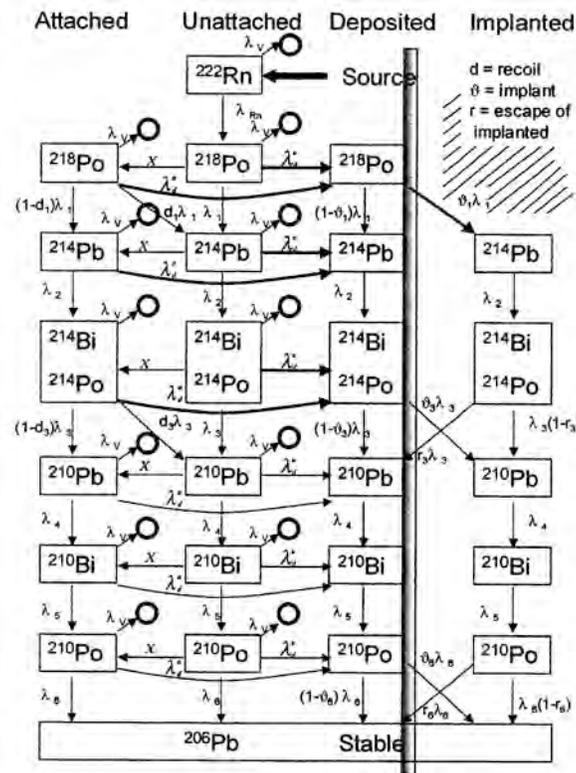
Figure 1: Schematic representation of process and parameters that affect airborne radon progeny activity size concentrations
