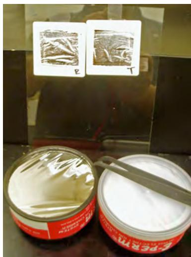
Figure 4 Track registration detectors (top) and electret ion chambers for measuring surface deposited radon and thoron progeny.
