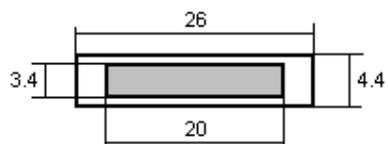
Figure 1. Dimensions of the polyethylene capsule used for preparation of NIST radon standard reference materials.
