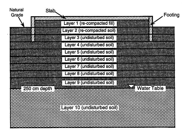
Fig. 1. Soil profiles defined for radon entry simulations.
