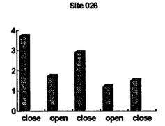
While lower radon levels under open stack conditions were observed in quite a few of the early test houses, in many of the cases the fluctuations were either so small that they are not conclusive, or the number of test rounds to date is small enough that statements on performance would be premature.
