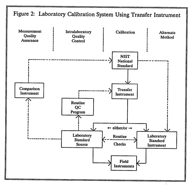
In general, the uncertainty of the final measurements increase as the number of steps from the National Standard increase. However, by using very accurate and precise instruments as Transfer Standards, this uncertainty can be kept well below the inherent uncertainty of the field instrument under calibration. Again it should be emphasized that
