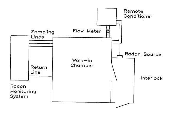
Figure 1. Layout of Bowser-Morner Radon Chamber
