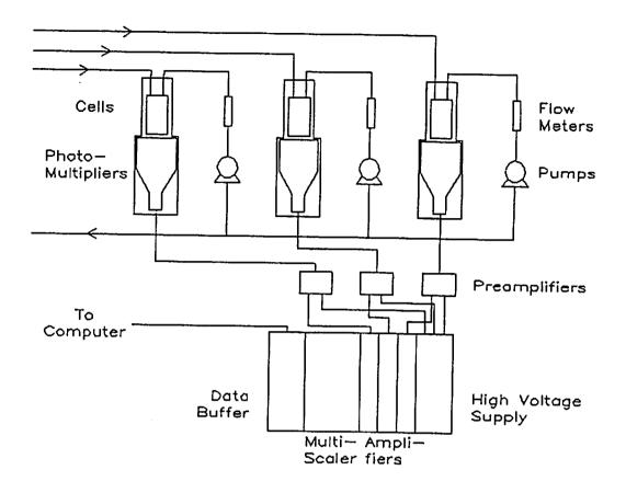
Figure 2. Diagram of Radon Monitoring System
