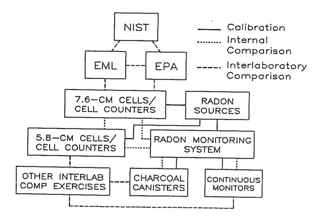
Figure 3. Diagram of Calibrations and Comparisons
