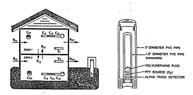
Figure 1. Schematic Representation of the Experimental System Used to Determine Multizone Radon Source Rates (after Kunz 1989)
