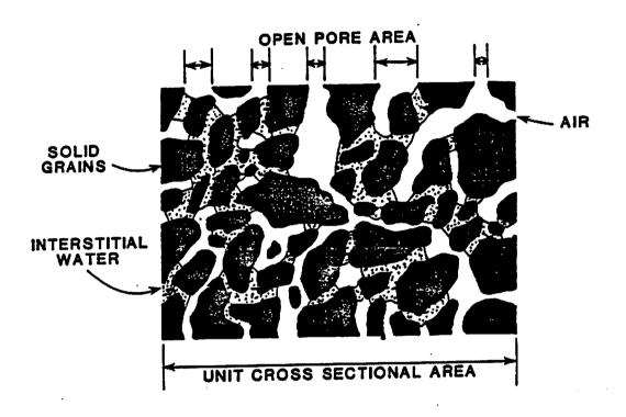
FIGURE 2. Volume of unsaturated porous material radium is in the solid grains and interstitial water.
