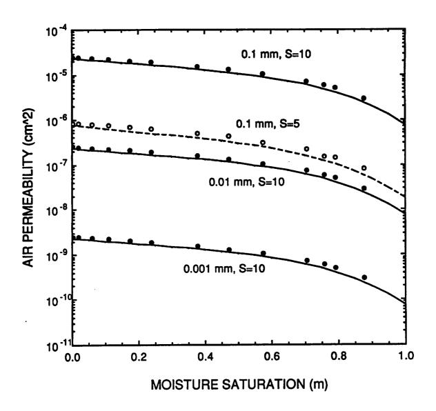
Figure 4. Air permeability for various soil types. Data points are model calculations. Curves are correlation values. Geometric mean particle diameters, and geometric standard deviations, S, are given for each soil type.
