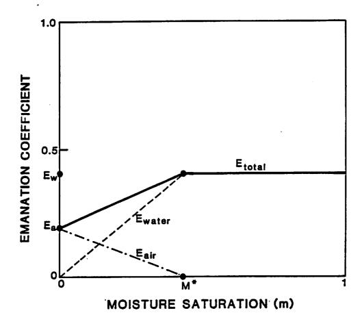
FIGURE 3. Components of the emanation coefficient as a function of moisture.
