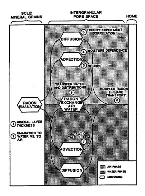
FIGURE 1. Physical mechanisms of radon generation and transport.
