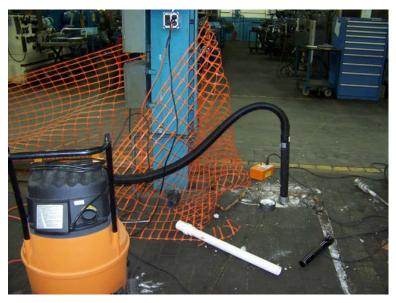
Figure 8 Sub-Slab Communication Test
