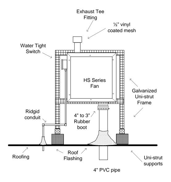
Figure 49, Roof Top Installation Detail of HS Blower
