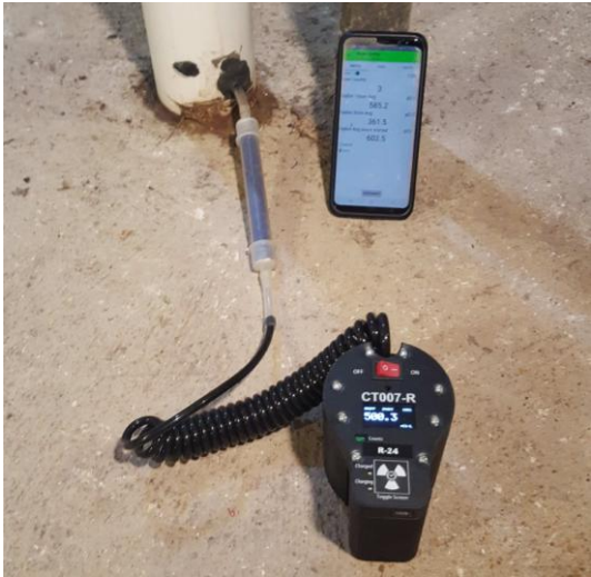
Figure 38: Using CT007-R to measure ASD pipe
