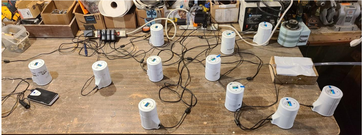
Figure 25: Diffusion of 175 pCi/l @ 20 LPM Flow
