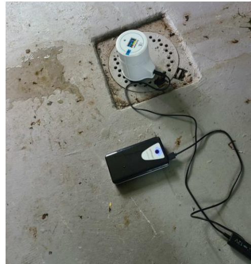
Figure 31: Floor drain measurement
