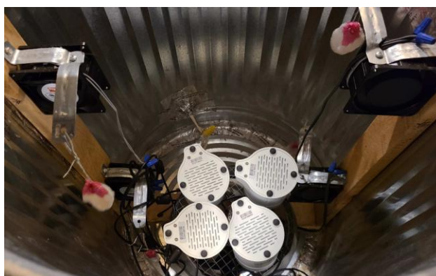
Figure 43: Ecotrackers in Thoron chamber with thoron mantles and circulating fans
