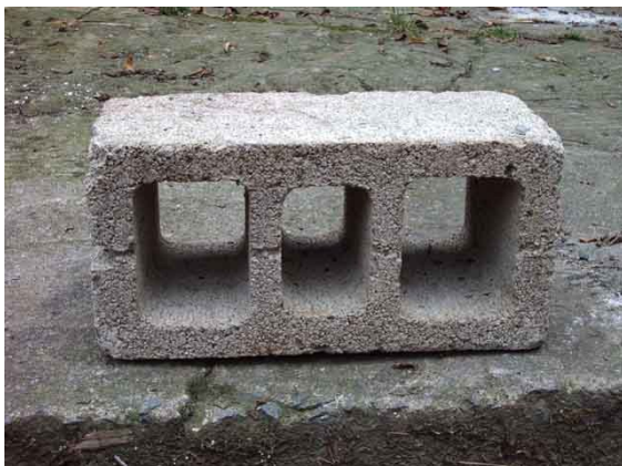
Photo 1 – Hollow Concrete Block
