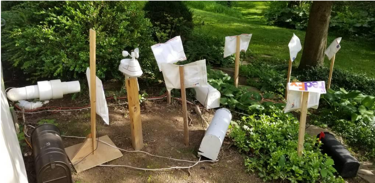
Figure 12: CRM and weather station placement in ASD exhaust stream
