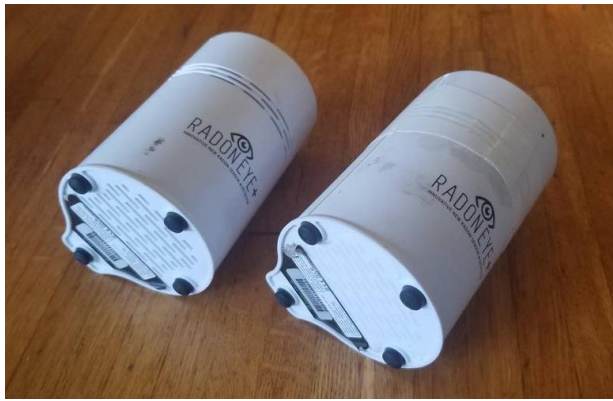
Figure 7: Radon Eye un-taped and taped to delay thoron entry
