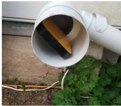
Figure 8: Corentium Pro installed in exhaust piping
