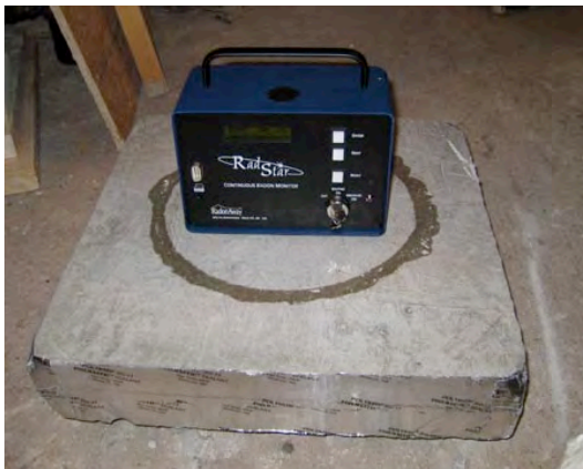
Figure 11 – RS800 sealed under 9.6 Liter Accumulator for Mixed Slab
