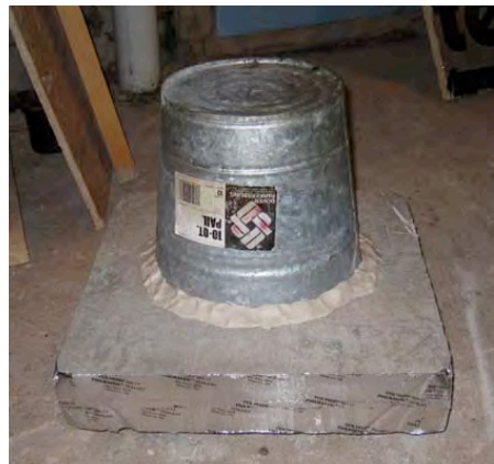
Figure 11 – RS800 sealed under 9.6 Liter Accumulator for Mixed Slab
