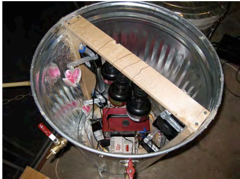
Figure 6 - 114 liter Thoron Chamber using Aladdin mantles & fans
